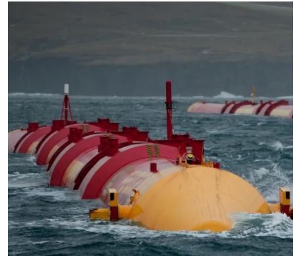
Wave energy converter (WEC) transforms the kinetic energy of ocean waves into electricity
